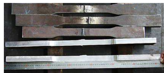
Figure 5 - Butt weld specimens (thickness range between 50 and 75 mm)
